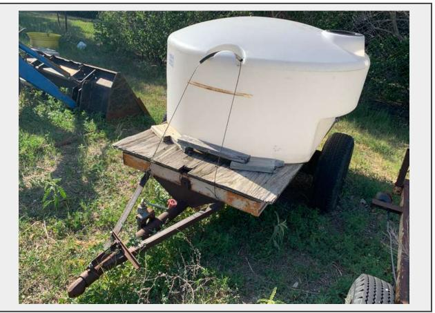
**Dimensions** 4' x 7'- 9" **Deck** Plywood **Hitch Type** 2" Ball Receiver
