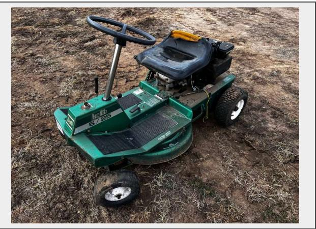
Make LongLife Model 47-215-10 Engine Magnetron Briggs & Stratton Horse Power 5.0 Tire Size 13x5.00-6
