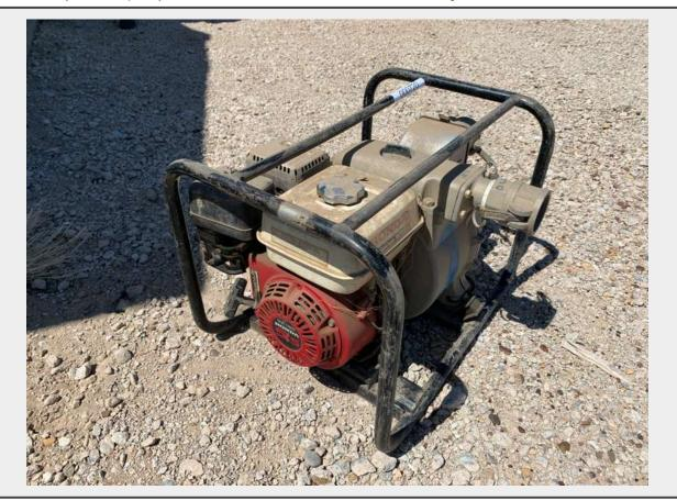
Make Honda Model WT20X Horse Power 5.5HP Fuel Type Gasoline
