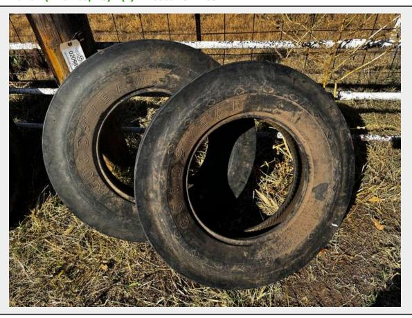
Make Goodyear Model Drill Rib Tire Size 7.50-20
